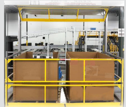
POWERED OVERHEAD SAFETY GATE
